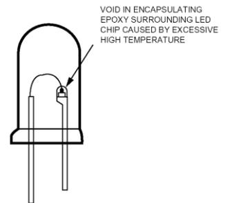
**Incorrect assembly procedures:** Overheating of the LED lamp device by excessive soldering during assembly can cause breakage of the anode-to-cathode wire bond. More significantly, inappropriate bending of the LED leads during assembly causes stresses in the lead frame which are transmitted to the encapsulating epoxy, causing it to crack. Importantly, this cracking shows up not immediately, but later, as a latent field failure.
