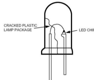
**Long-term exposure to condensing moisture** can cause the epoxy encapsulation of the LED to deteriorate. This will lead to catastrophic failure by corroding the top contact on the LED chip or by breaking the anode-to-cathode bonding wire, apart from decomposing the epoxy over time.
